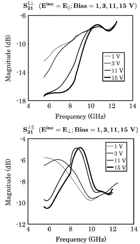
Fig. 4. (top) Axial incidence cross-polarization transmission,  $S_{21}^{\parallel\perp}$ ; (bottom) Perpendicular incidence cross-polarization transmission,  $S_{21}^{\perp\parallel}$ .
