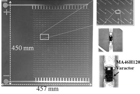
Fig. 2. Fabricated Sample top side loaded with MA46H120 varactor diodes.
