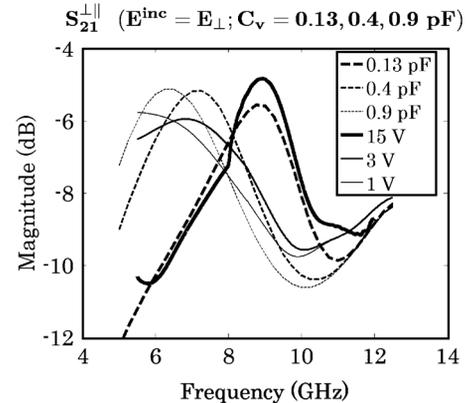
Fig. 5.  $S_{21}^{\perp\parallel}$ : measured (solid lines) against HFSS simulated (dashed lines).
