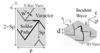
Fig. 1. Chiral array in one period with design parameters: 9 mm pitch ( $P$ ); 6 mm spacing ( $Sp$ ); 0.3 mm trace width ( $w$ ); 2.2 dielectric constant of substrate; 3.2 mm substrate thickness ( $d$ ); ( $C_v$ ) 0.13–0.9 pF capacitance range.
