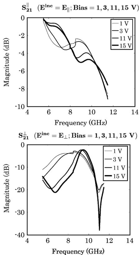
Fig. 6. (top) Axial incidence total transmission,  $S_{21}^{\parallel}$ ; (bottom) Perpendicular incidence total transmission,  $S_{21}^{\perp}$ .
