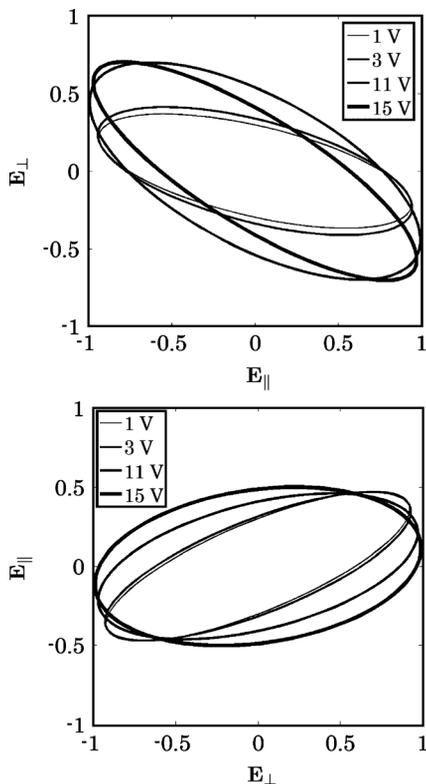
Fig. 7. (top) Transmitted wave polarization in axial incidence,  $E_{\perp}$  vs.  $E_{\parallel}$  and (bottom) in perpendicular incidence,  $E_{\parallel}$  vs.  $E_{\perp}$ , both at 9 GHz.
