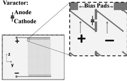
Fig. 3. Varactor (top) side of the helix array. Individual helices themselves are used as bias lines.
