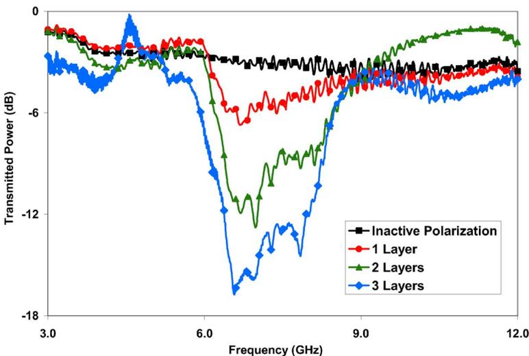
FIG. 5. The transmitted power through one, two, and three layers of the hand-fabricated FDR. Also shown, is the transmission when incident wave is polarized in such a way not to interact with the FDRs.
