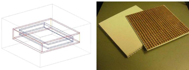
FIG. 3. (left) Schematics of a folded-double resonator. (right) Samples made from adhesive copper tape.
