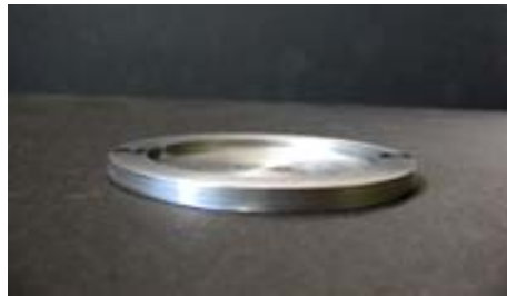
Figure 1. Un-deformed DH-36 steel plate
