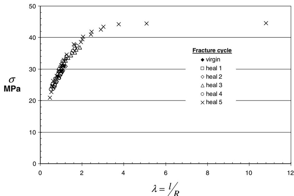
Fig. 5. Stress vs. crack length data of five fracture–healing cycles for specimen 1. All healing treatments for specimen 1 consisted of applying pressure while heating to 85 °C for 10 h followed by heating to 95 °C for 3 h with no applied pressure.
