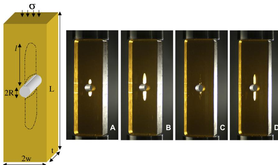
Fig. 4. Left: schematic of DCDC sample geometry. Dotted lines represent the location of the pre-crack and subsequent crack extension. Right: fracture and healing sequence of a single sample. (A) Virgin sample with hole and pre-cracks visible; (B) sample after first fracture event; (C) sample after first healing treatment; (D) sample after second fracture event.
