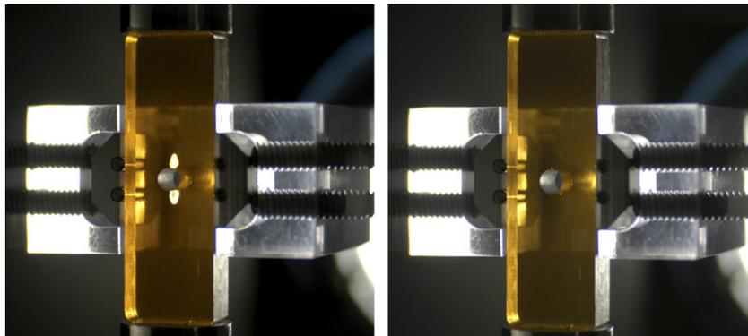
Fig. 3. Lateral confining fixture attached to specimen to create pre-crack. Left: specimen prior to axial compression with small razor notches visible at upper and lower crowns of central hole. Right: application of axial compression initiates cracks which propagate from razor notches and are arrested at a length of  $\sim 1.8\text{ mm}$ , which forms the pre-existing crack for subsequent fracture-toughness measurement.
