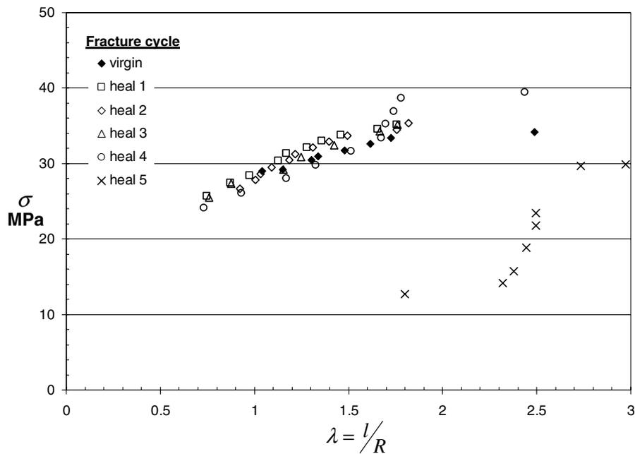
Fig. 8. Initial portion of stress vs. crack length data shown in Fig. 7 for specimen 2.
