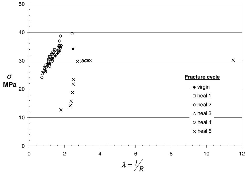
Fig. 7. Effect of different healing treatments on the resulting fracture strength of specimen 2.
