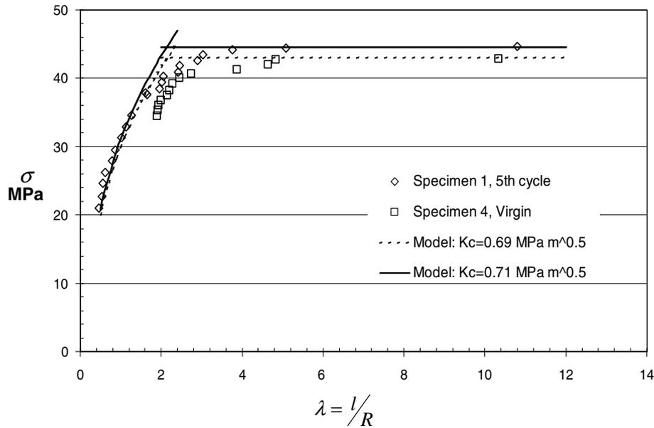
Fig. 11. Fracture into virgin polymer for specimen 4 in relation to model prediction with  $K_c = 0.692 \text{ MPa m}^{1/2}$ , and specimen 4 after five cycles of fracturing and healing with  $K_c = 0.716 \text{ MPa m}^{1/2}$ .
