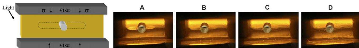
Fig. 12. Illustration of in-situ photos of representative healing treatment at 85 °C. Left: orientation of sample with respect to camera. Right: sequence of photos during treatment at 85 °C. (A) Time 0; (B) 2 min; (C) 4 min; (D) 15 min.
