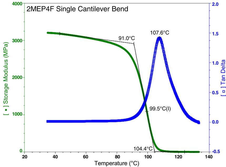
Fig. 2. Dynamic mechanical analysis of 2MEP4F polymer cycled at 1 Hz and heated at  $3\text{ }^{\circ}\text{C min}^{-1}$ .
