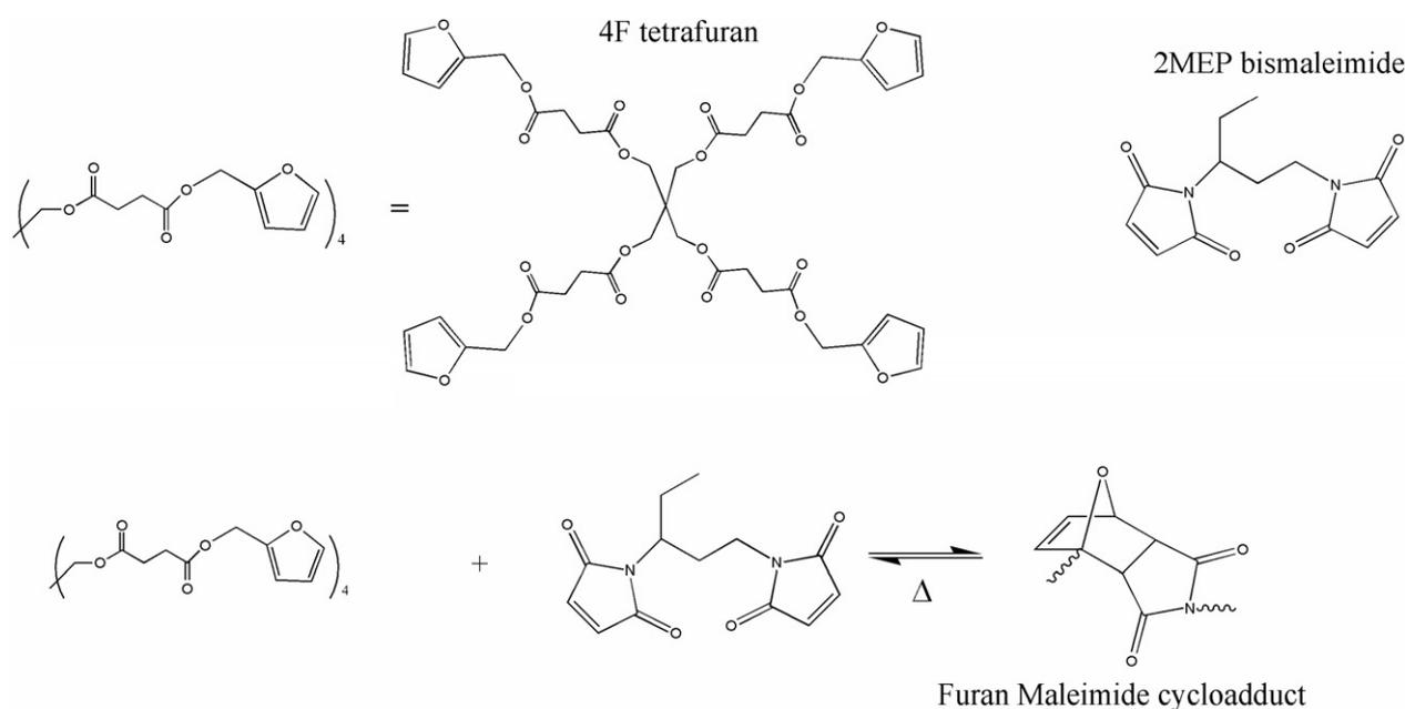
Fig. 1. The polymer consists of a multifuran molecule combined in stoichiometric ratio with a multimaleimide molecule to form 2MEP4F cycloadduct.
