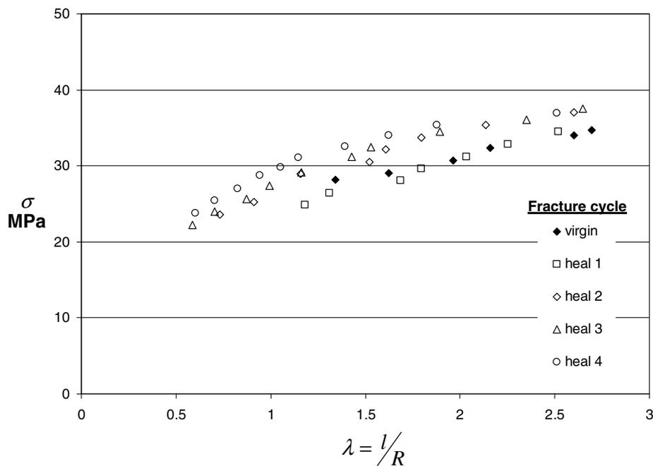
Fig. 10. Initial portion of stress vs. crack length data shown in Fig. 9 for specimen 3.
