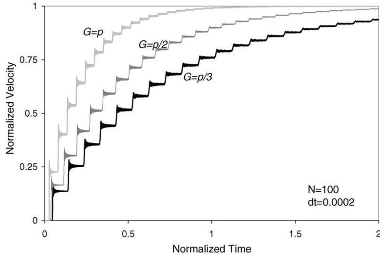
Fig. 2. Normalized particle velocity (velocity/ $V_0$ ) in the rear plate for indicated values of the shear modulus,  $G$ . In the absence of release waves reflecting off the free faces of the steel plates, the final velocity would approach  $V_0$  regardless of the value of the shear modulus, if there is no interface slip or other material failure. Normalized time = actual time/( $l/V_0$ ).
