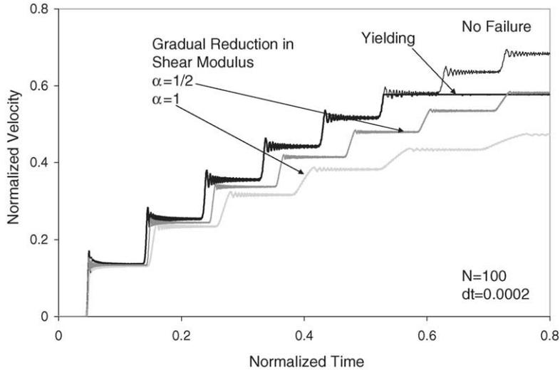
Fig. 4. Effect of stiffness degradation or yielding (interface slip) on the rear plate particle velocity.
