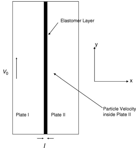
Fig. 1. A thin elastomer layer is sandwiched between two thick steel plates and uni-axially pre-strained. A shear wave with particle velocity  $V_0$  traveling through plate I in the  $x$ -direction, impacts the elastomer. The shear velocity at a typical point inside the rear plate is calculated based on the properties of the elastomer.
