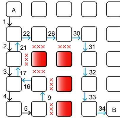
Figure 4. Example of developed message routing algorithm for our nearest neighbor mesh network.
