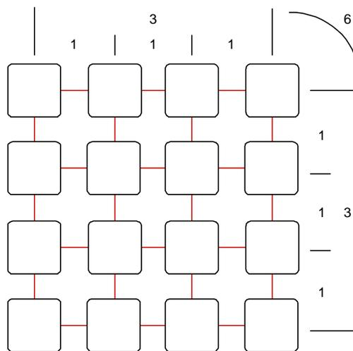
Figure 3. Nearest-neighbor mesh network. A PE's communication is restricted to its nearest neighbors only. For communication with other nodes, a message passing protocol must be developed. The numbers represent the effective network distance, thus to pass a message from the PE in the upper left to the PE in the bottom right takes 6 steps. This network can easily be improved by connecting the first and last PE in each row and column making it a torus network.
