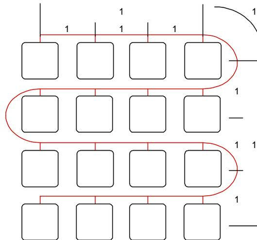
Figure 2. Global Bus network. Similar to the mesh network in that all PEs are peers, but each PE is connected to every other PE via a common bus, as opposed to individual connections. The numbers in the figure represent the network distance between two PEs. Nearest neighbors are at a distance of 1 as are the two PEs in the same at opposite ends of a row or a column. The number in the upper right indicates the network distance between the PEs at (1,1) and (4,4); in this case it is also 1.
