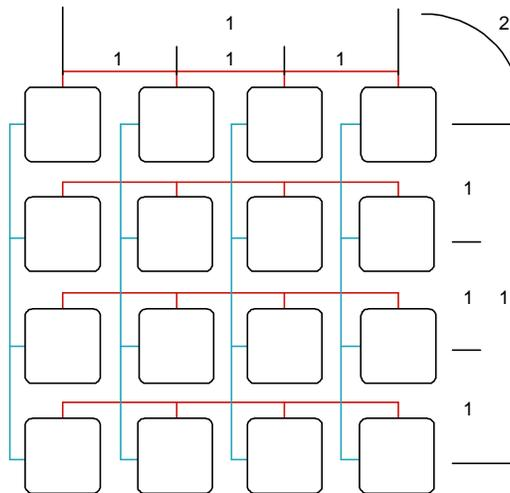
Figure 5. Row-Column Bus Array. Each row and column has its own bus to pass data. This significantly speeds up average communication over global bus network (Figure 2) by allowing simultaneous communications over the network while only increasing the network distance to 2.
