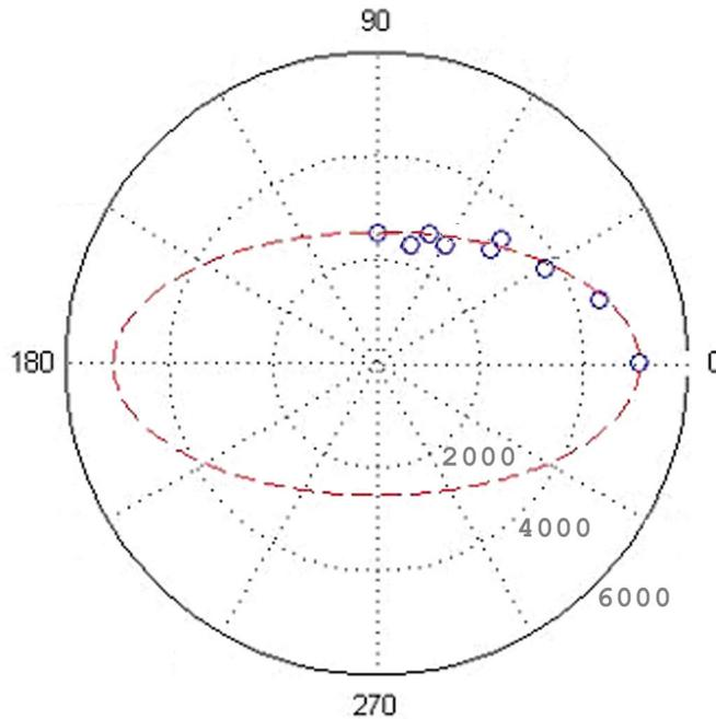
Figure 1. Acoustic wave velocity (m/s) measured in unidirectional FRP plate – made using pencil graphite break test and collinear ultrasonic transducers.
