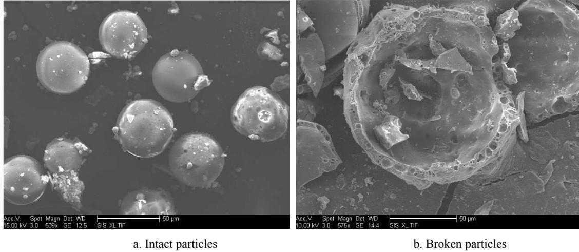
Figure 1. SEM images of fly ash prior to casting in polyurea.
