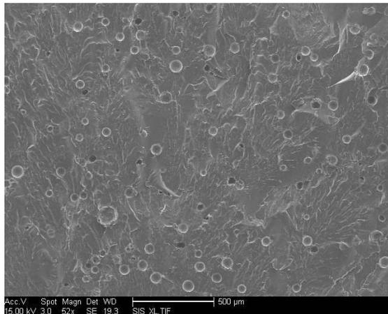
Figure 3. Fractographs of composites filled with 5% small size fly ash (<math><74\mu\text{m}</math>).
