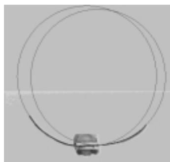
FIG. 6-D. Circle fitted to deformed sample; Flemion-based IPMC in  $K^+$ -form (FL4K-00) with ethylene glycol as solvent; 1.5 volt; end of bending toward anode before shorting (474 Seconds)
