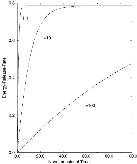
Fig. 5. Dependence of the nondimensional energy-release-rate  $\mathcal{E}$  on the nondimensional time for a bridged crack in an isotropic material, under uniform external load and indicated values of  $l = \pi(1 + \kappa)K_0c/2\mu T_0$ .
