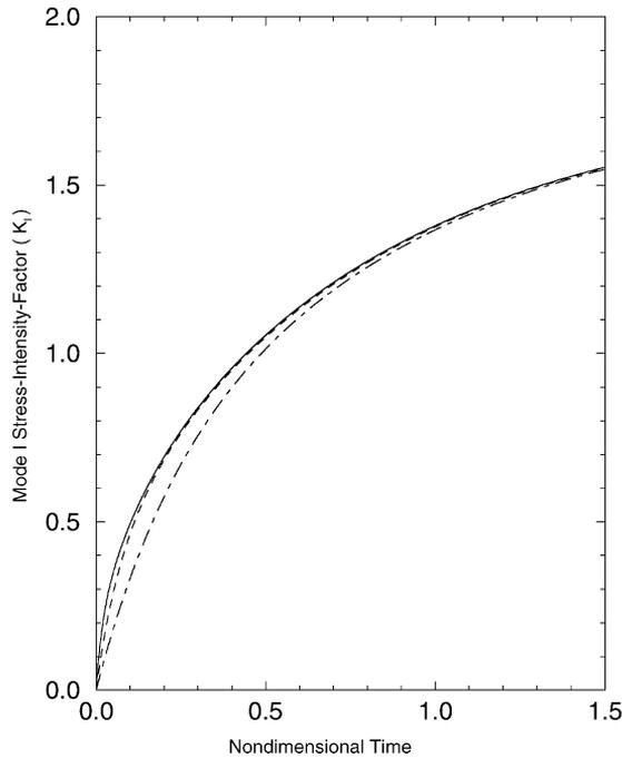
Fig. 1. Nondimensional mode I stress-intensity-factor  $K_I$  vs. the nondimensional time  $\hat{t}/T_0$  for a bridged crack in an isotropic material, under uniform external load;  $l = \pi(1 + \kappa)K_0c/2\mu T_0 = 1$ ,  $\Delta t = 0.001$ , and  $N + 1 = 4$  (dot-dashed), 8 (dashed), and 16, 32, 48, and 64 (solid) curves, respectively.
