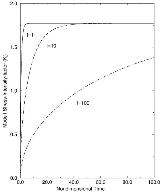
Fig. 3. Dependence of the nondimensional mode I stress-intensity-factor on the nondimensional time for a bridged crack in an isotropic material, under uniform external load and indicated values of  $l = \pi(1 + \kappa)K_0c/2\mu T_0$ .
