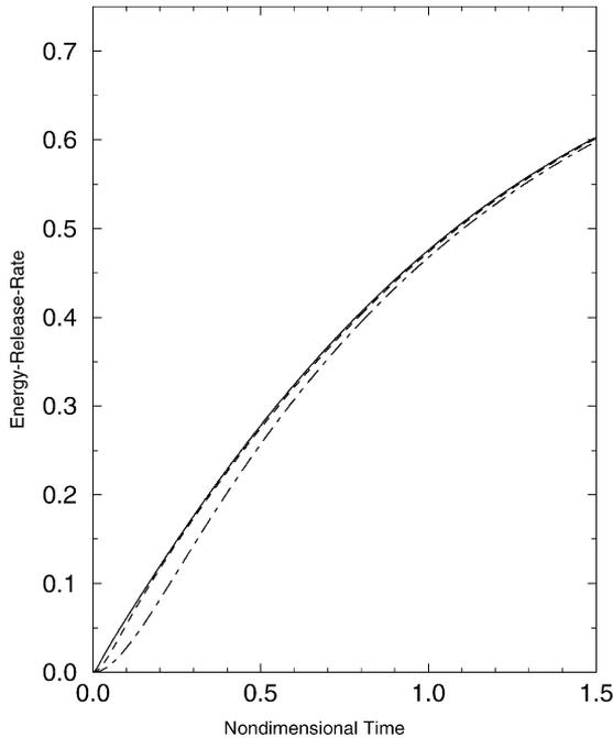
Fig. 2. Nondimensional energy-release-rate  $\mathcal{E}$  vs. the nondimensional time  $\hat{t}/T_0$  for a bridged crack in an isotropic material, under uniform external load;  $l = \pi(1 + \kappa)K_0c/2\mu T_0 = 1$ ,  $\Delta t = 0.001$ , and  $N + 1 = 4$  (dot-dashed), 8 (dashed), and 16, 32, 48, and 64 (solid) curves, respectively.
