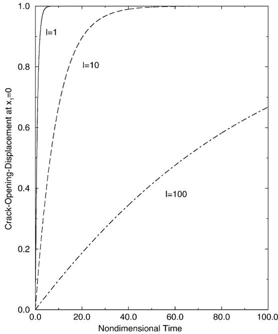
Fig. 4. Dependence of the nondimensional crack-opening-displacement at  $x = 0$  on the nondimensional time for a bridged crack in an isotropic material, under uniform external load and indicated values of  $l = \pi(1 + \kappa)K_0c/2\mu T_0$ .
