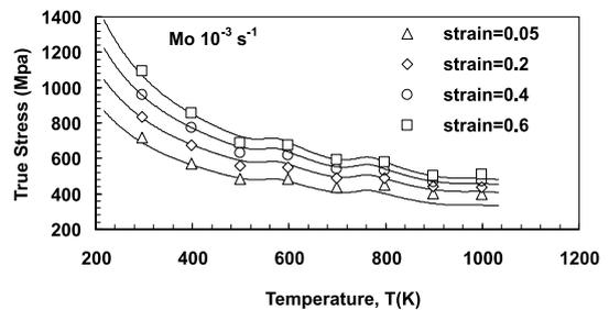
Fig. 2. Flow stress vs temperature curves for molybdenum at indicated plastic strain (symbols: experimental, solid lines: theoretical).
