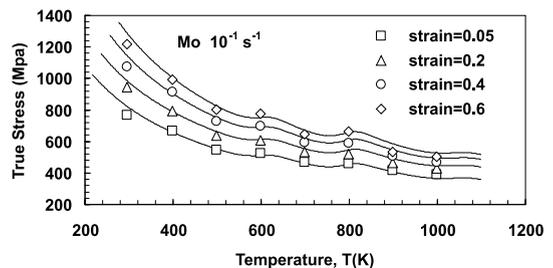
Fig. 3. Flow stress vs temperature curves for molybdenum at indicated plastic strains (dotted lines: experimental, solid lines: theoretical).
