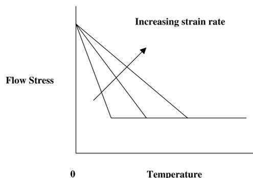
Fig. 8. Sketch of the dependence of flow stress on temperature at different strain rates under the framework of classical theory of thermal activation.
