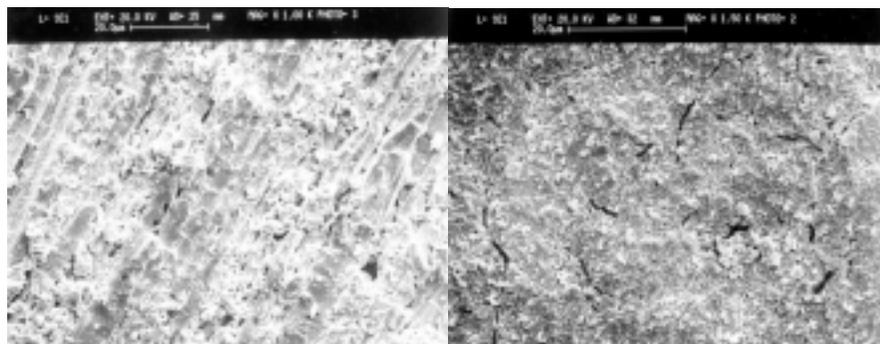
**Figure 6:** Scanning electron microscopic photos of IPMC surfaces, showing microcracks on Nafion- (left) and on Flemion- (right) based IPMCs.
