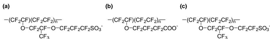
**Figure 2:** Perfluorinated ionomers used in IPMC manufacture include (a) Aciplex, (b) Flemion, and (c) Nafion.
