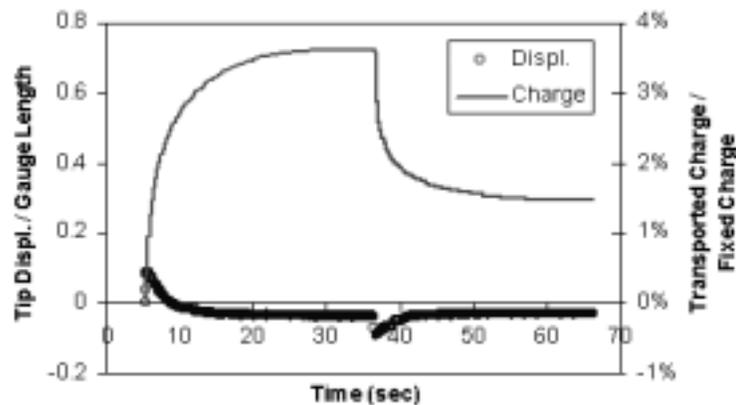
**Figure 12:** Tip displacement and accumulated charge versus time for a Nafion-based IPMC in  $\text{Na}^+$ -form, with 1.5V DC applied and then shorted.
