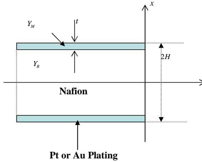
**Figure 10:** Edge-on diagram of IPMC used in modeling force output.
