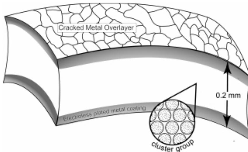
**Figure 1:** IPMC schematics indicating surface morphology, interface, and cluster structure.
