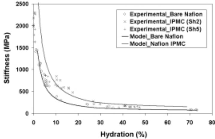
**Figure 16:** Uniaxial stiffness (Young's modulus) of bare Nafion 117 (lower data points and the solid curve, model) and an IPMC (upper data points and light curve) in the Na<sup>+</sup>-form versus hydration water.
