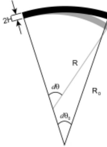
**Figure 11:** Pure bending of an element of an IPMC strip corresponds to a change in the local radius of curvature.
