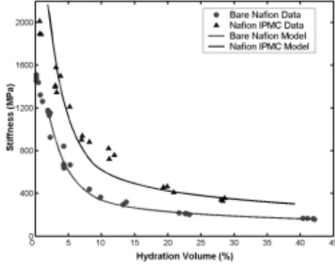
**Figure 9:** Stiffness versus hydration of Flemion ionomer (lower data points and the solid curve) and IPMCs (upper data points and the solid curve) in Cs+-form.
