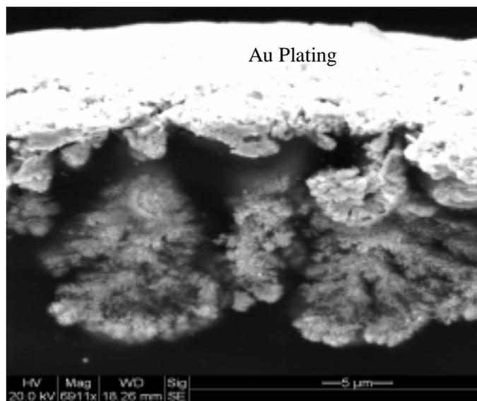
**Figure 5:** Cross section of a typical Au-plated Flemion-1.44, showing dendritic structure of gold electrodes.
