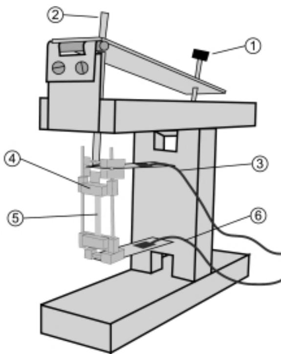
**Figure 7:** Diagram of mini-load frame. (1) Force adjuster, motorized; (2) force arm; (3) displacement gauge; (4) sample clamps; (5) IPMC sample; (6) load-displacement gauge.
