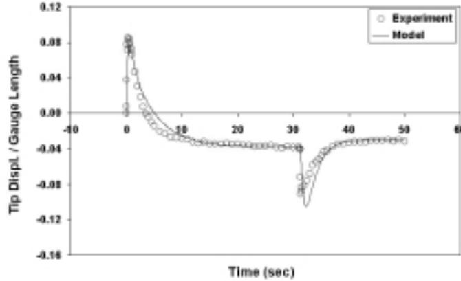
**Figure 15:** Tip displacement of a 15mm cantilevered strip of a Nafion-based IPMC in  $\text{Na}^+$ -form, subjected to 1.5 V step potential for about 32 seconds, then shorted; the heavy solid curve is the model and the geometric symbols are experimental points.
