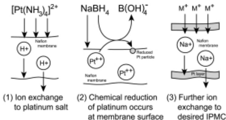
**Figure 3:** Scheme for IPMC fabrication: (1) ion exchange with noble metal salt; (2) reduction of metal at surface; (3) ion exchange with desired cation.
