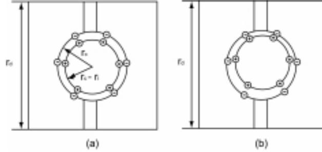
**Figure 17:** Schematic representation of IPMC clusters: (a) an arrangement of ions into dipoles within cluster, and (b) a dipole induced by imposed bending curvature.
