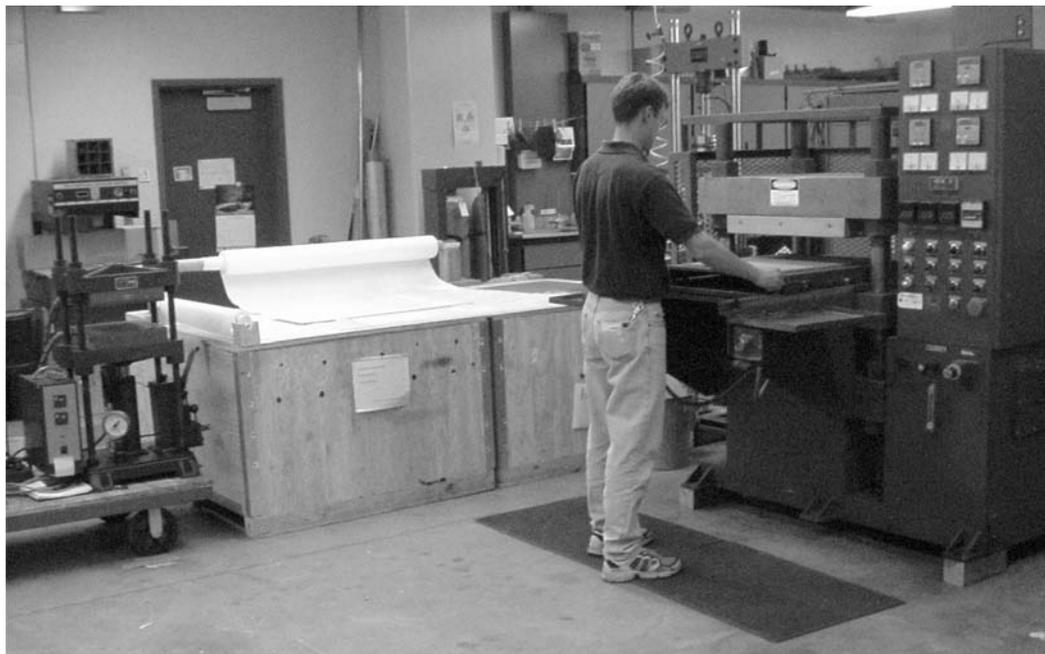
Figure 12.3 (Top) Schematic of two-dimensional thin wire array. One hundred micrometer wires are periodically embedded between composite laminates with layup jig to yield a processed fiberglass/epoxy laminate with array visible inside. (Bottom) Laminating hot presses for processing composite panels.
