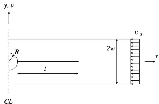
**Fig. 6** Schematics and dimensions of the DCDC model
