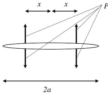
**Fig. 5** Representation of a slit crack with symmetric concentrated loads
