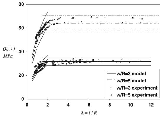
**Fig. 10** Axial load versus normalized crack length for  $w/R = 3$  and  $5$ : The solid and dashed curves represent the model results for the indicated values of  $w/R$ , using the critical stress intensity factors  $K_{IC} = 0.71 \text{ MPa}\sqrt{m}$  and  $K_{IC} = 0.64, 0.78 \text{ MPa}\sqrt{m}$ . The initial curved segment is the short-crack solution and the flat line is the asymptotic long-crack solution
