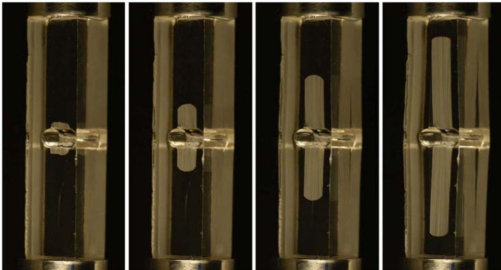
**Fig. 2** Picture sequence, from left to right, of advancing crack. The third picture from the left shows the sample loaded well into the plateau regime. Sample is viewed from same perspective as shown in Fig. 1
