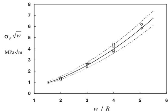
**Fig. 8** Plateau stress vs.  $w/R$  ratio. The circles are the experimentally measured values. The solid curve represents the model result for a critical stress intensity factor of  $K_{IC} = 0.71 \text{ MPa}\sqrt{m}$ , while the dashed curves are for a 10% variation, i.e.,  $K_{IC} = 0.64, 0.78 \text{ MPa}\sqrt{m}$
