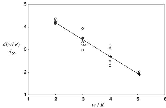
**Fig. 7** Normalized values of  $d(w/R)$  with respect to the theoretical prediction in an infinite plate
