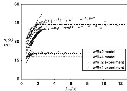
**Fig. 9** Axial load versus normalized crack length for  $w/R = 2$  and 4: The solid and dashed curves represent the model results for the indicated values of  $w/R$ , using the critical stress intensity factors  $K_{IC} = 0.71 \text{ MPa}\sqrt{m}$  and  $K_{IC} = 0.64, 0.78 \text{ MPa}\sqrt{m}$ . The initial curved segment is the short-crack solution and the flat line is the asymptotic long-crack solution
