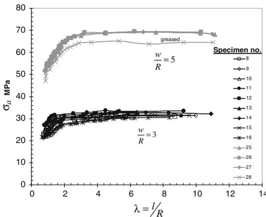
**Fig. 4** Experimental data for specimens with  $w/R$  ratios 3 and 5
