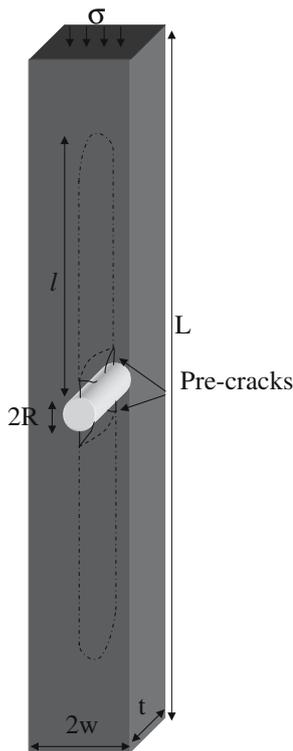
**Fig. 1** DCDC specimen with central hole. Solid lines emanating from the crowns of the hole indicate the shape and location of the initial pre-cracks. Upon loading, pre-cracks connect and propagate (dotted lines) towards the direction of applied compression
