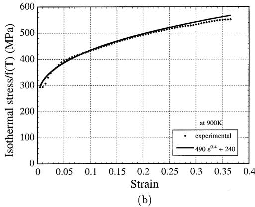
Fig. 5. Isothermal flow stress of (a) Ta and (b) Ta–2.5%W, at 900 K–3000/s, fitted to Eq. [16]. Here, it is assumed that the flow stress at 900 K–3000/s is athermal.
