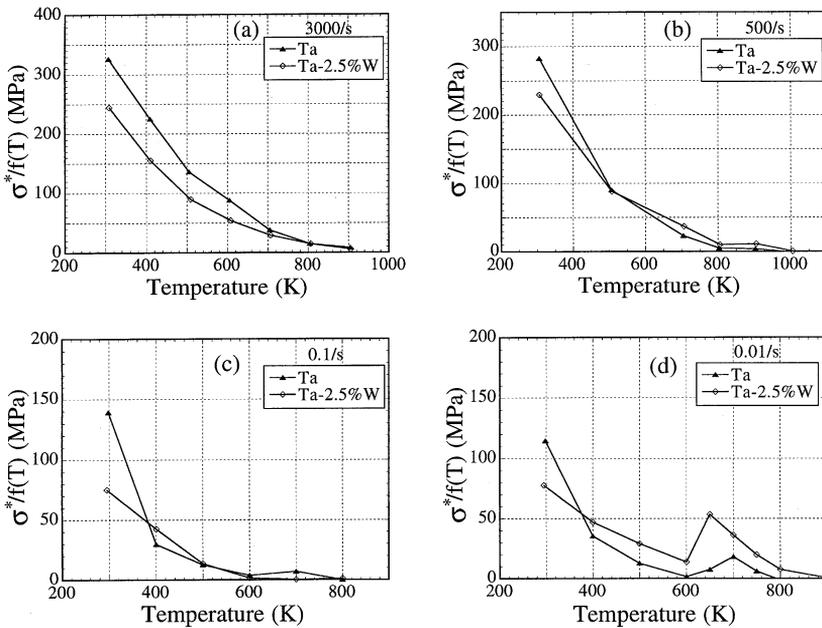
Fig. 8. Flow stress as a function of temperature, comparing Ta and Ta–2.5%W at (a) 3000/s, (b) 500/s, (c) 0.1/s, and (d) 0.01/s.
