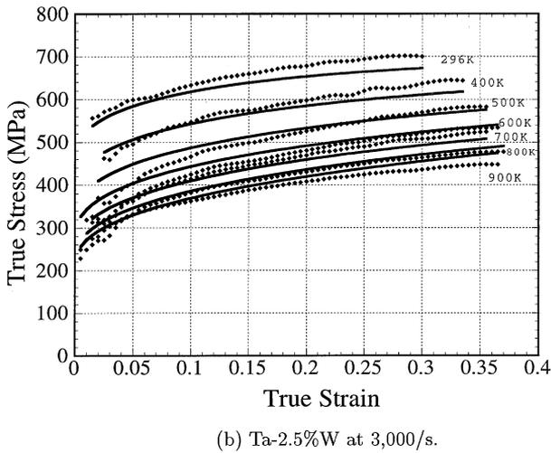
Fig. 6. Experimental flow stress as function of strain, compared to calculated values using Eq. (17).
