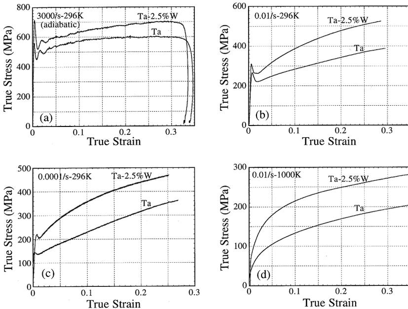
Fig. 7. Stress–strain plot, comparing Ta and Ta–2.5%W at (a) 3000/s–296 K, (b) 0.01/s–296 K, (c) 0.0001/s–296 K, and (d) 0.01/s–1000 K.
