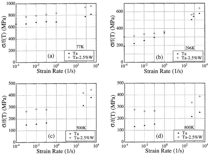
Fig. 9. Flow stress as a function of strain rate, comparing Ta and Ta–2.5%W at (a) 77 K, (b) 296 K, (c) 500 K and (d) 800 K.
