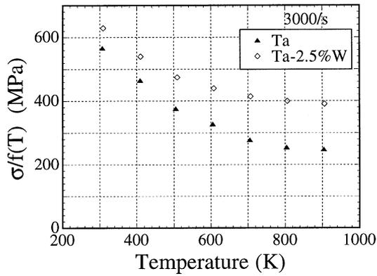
Fig. 3. Plot of  $\sigma/f(T)$  vs.  $T$  at 0.05 strain at 3000/s for Ta and Ta–2.5%W.
