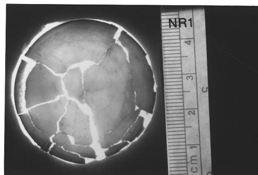
FIG. 14. Specimen recovered in the normal recovery experiment where only circular plates were used.
