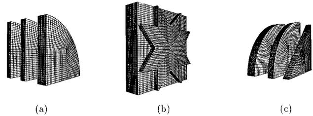
FIG. 4. Normal recovery configurations: (a) all circular plates; (b) star-shaped flyer with square plates; (c) square-shaped flyer with circular plates.
