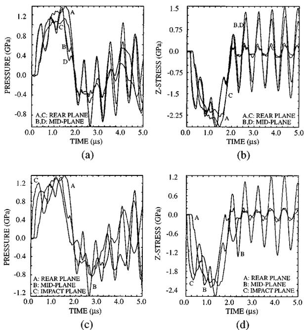
FIG. 9. Pressure–shear recovery configuration—pressure and longitudinal compression histories: (a),(b) square-shaped second flyer with circular plates; (c),(d) two squares—a second flyer and a square momentum trap.
