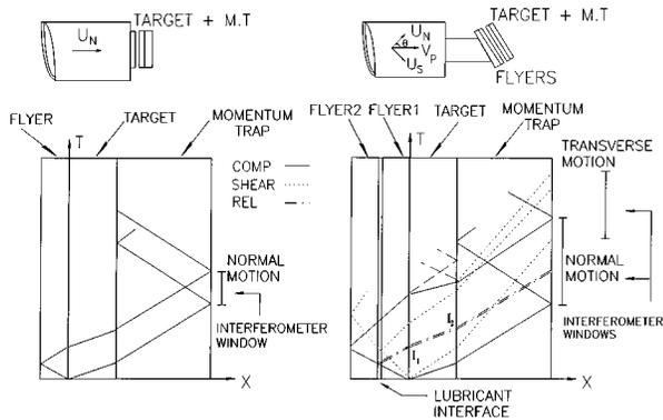
FIG. 1. Time–distance diagrams for normal and pressure–shear recovery configurations.
