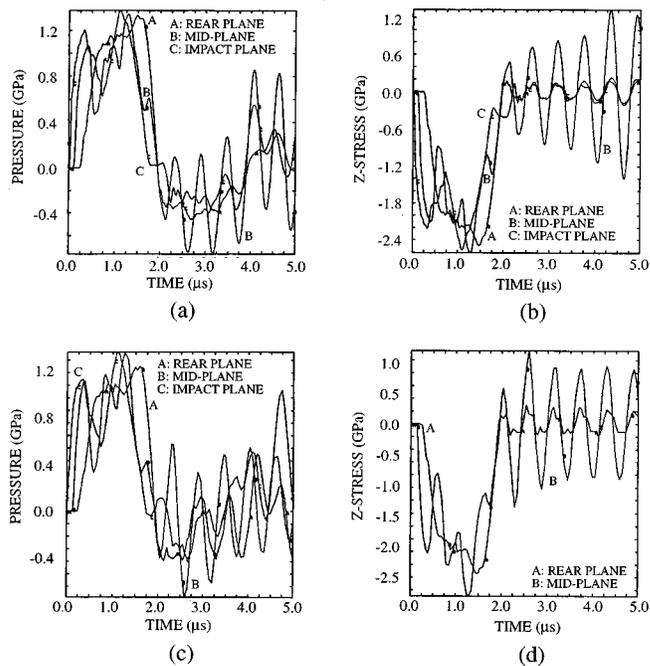
FIG. 10. Pressure–shear recovery configuration—pressure and longitudinal compression histories: (a),(b) star-shaped second flyer— $\pi/4$  type and square plates; (c),(d) square-shaped second flyer with critical planes on the circular specimen.
