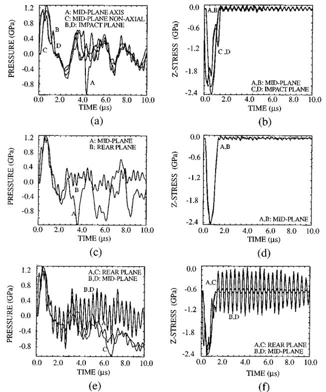
FIG. 5. Pressure and longitudinal stress histories in normal impact recovery configurations: (a),(b) all circular plates; (c),(d) star-shaped flyer— $\pi/4$  type and square plates; (e),(f) square-shaped flyer with circular plates.
