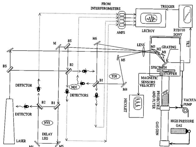
FIG. 2. Layout of a pressure–shear recovery experiment.
