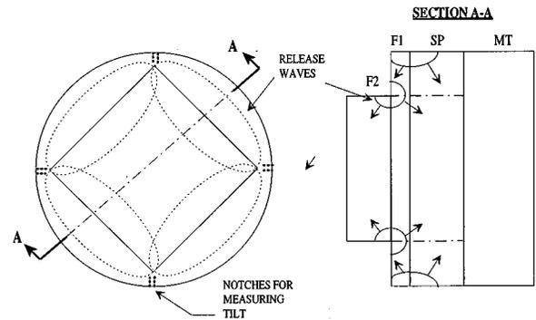
FIG. 3. New design employing a square second flyer for pressure-shear recovery configuration.
