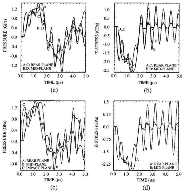
FIG. 8. Pressure–shear recovery configuration—pressure and longitudinal compression histories: (a),(b) all circular plates; (c),(d) star-shaped second flyer  $3\pi/4$  type.
