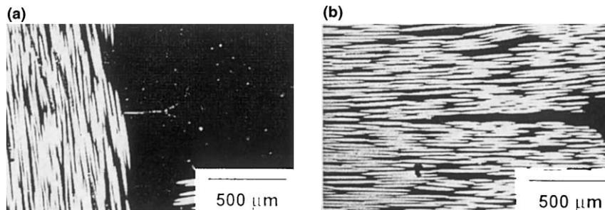
Fig. 7. Scanning electron micrographs of  $[0/90]_8^f$  coupons conditioned at 97 MPa. (a) 21°C; 3966 h; (b) 57°C; 1381 h.
