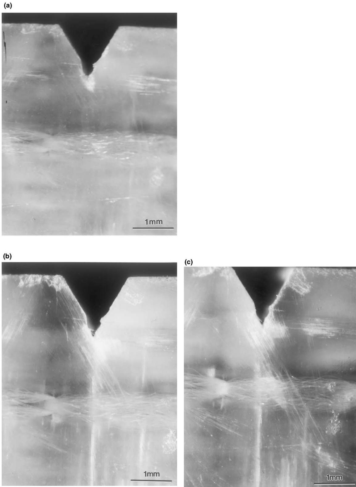
Fig. 2. Optical micrographs of  $[90/0]_{2s}$  coupon (a) prior to conditioning and of coupon conditioned at  $57^{\circ}\text{C}$  and  $145\text{ MPa}$  for (b) 300 h and (c) 900 h. Layup has chopped strand mat.
