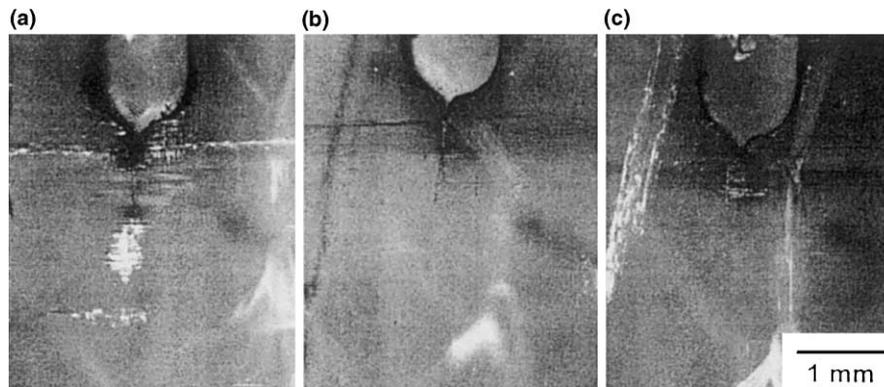
Fig. 4. Optical micrographs of  $[0/90]_8$  coupon conditioned at 57°C and 48 MPa for 1006 h. Depth from tool surface: (a) 0.4 mm, (b) 2.2 mm, and (c) 2.6 mm. Food coloring has been used to highlight damage.
