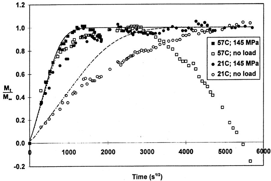
Fig. 9. Moisture absorption in notched  $[0/90]_{2s}$  coupons with chopped strand mat.
