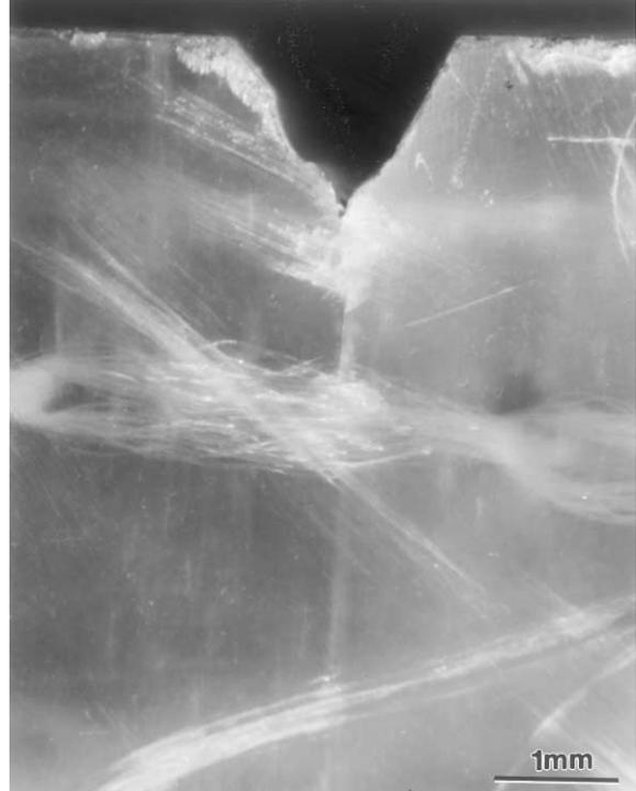
Fig. 1. Optical micrographs of  $[90/0]_{2s}$  coupon conditioned at 21°C and 145 MPa for (a) 2500 h, (b) 3000 h, and (c) 5500 h. Layup has chopped strand mat.
