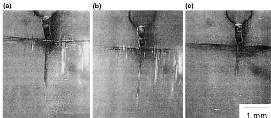
Fig. 5. Optical micrographs of  $[0/90]_8^f$  coupon conditioned at 21°C and 97 MPa for 3034 h. Food coloring has been used to highlight damage. Depth from tool surface: (a) 0.8 mm; (b) 1.0 mm; (c) 1.5 mm.
