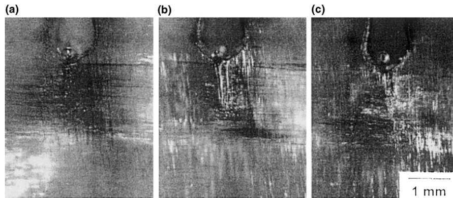
Fig. 6. Optical micrographs of  $[0/90]_8^f$  coupon conditioned at 57°C and 97 MPa for 1190 h. Food coloring has been used to highlight damage. Depth from tool surface: (a) 0.4 mm; (b) 0.7 mm; (c) 1.7 mm.
