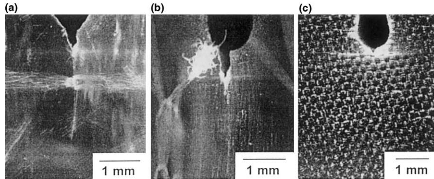
Fig. 8. Optical micrographs of coupons subjected to ambient conditions for 3000 h, (a) 145 MPa; layup is  $[90/0]_{2s}$ ; (b) 48 MPa; layup is  $[0/90]_8$ ; (c) 97 MPa; layup is  $[0/90]_8$ .
