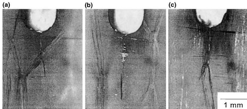
Fig. 3. Optical micrographs of  $[0/90]_8$  coupon conditioned at 21°C and 48 MPa for 3001 h. Depth from tool surface: (a) 0.6 mm, (b) 1.1 mm, and (c) 2.4 mm. Food coloring has been used to highlight damage.
