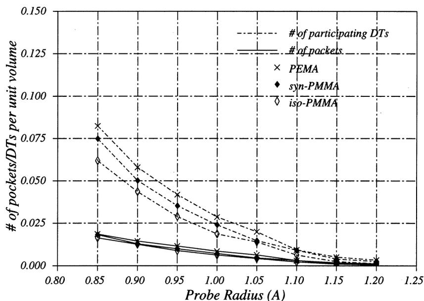
Fig. 11. Number of available volume pockets and DTs contributing to these pockets per unit volume for the acrylates.
