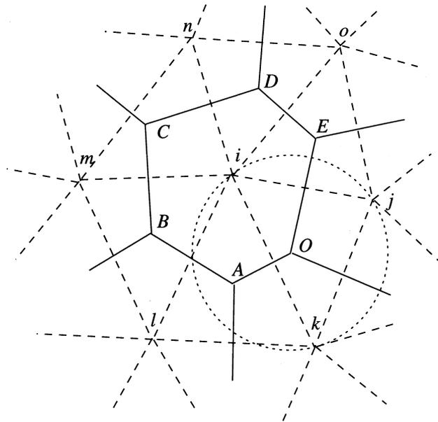
Fig. 1. Two-dimensional representation of Voronoi and Delaunay tessellations. The dashed lines show the Delaunay triangles and the solid lines show the Voronoi polygons.  $\Pi_i$  is given by OABCDE. The circum-circle centered at O for  $t(i, j, k)$  is also shown. Points  $i, j, k$  are contiguous and their Voronoi polygons meet at the point O.
