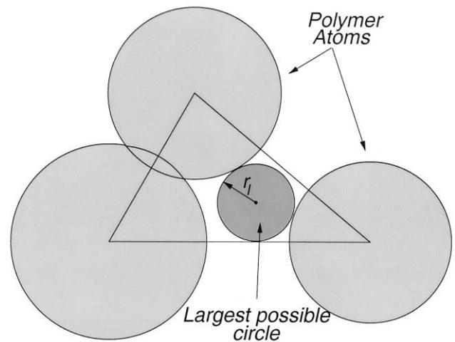
Fig. 4. Side of a DT. The darker circle represents the largest possible circle that can fit within the area of the face not occupied by the polymer atoms.
