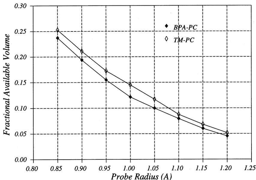
Fig. 8. Fractional available volume plots for TM-PC and BPA-PC.
