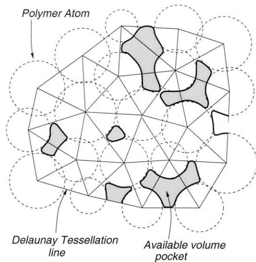
Fig. 3. Two-dimensional representation of available volume pockets.
