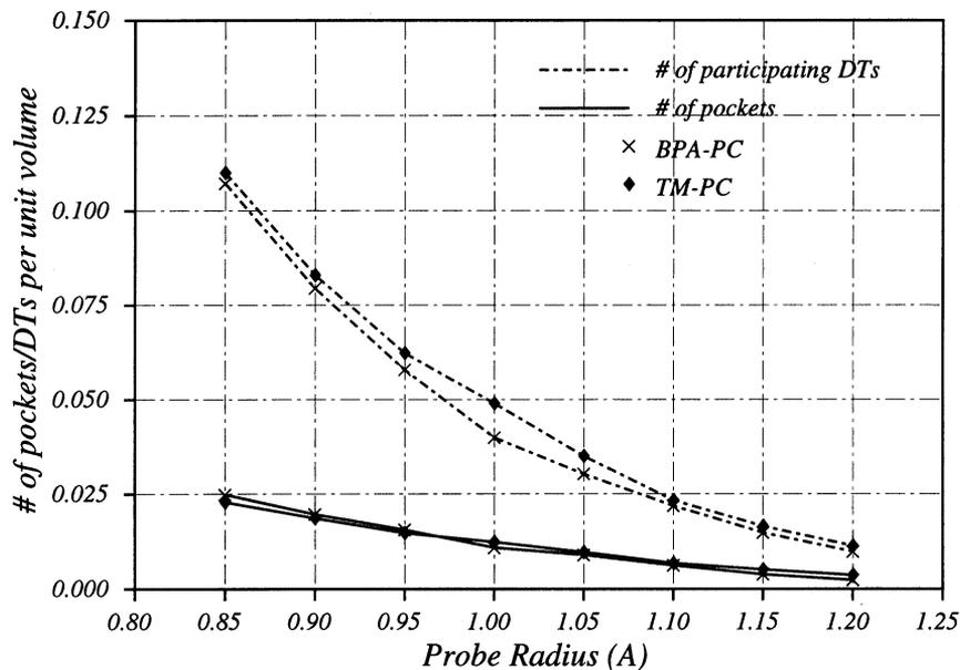
Fig. 10. Number of available volume pockets and DTs contributing to these pockets per unit volume for the polycarbonates.
