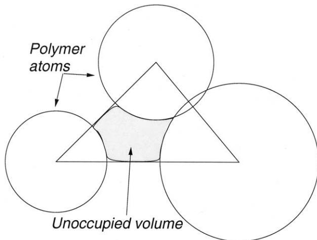
Fig. 2. Two-dimensional representation of unoccupied volume.
