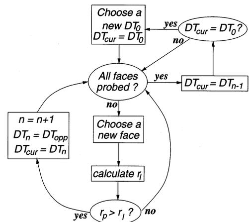
Fig. 5. Recursive algorithm used to evaluate each pocket of available volume.
