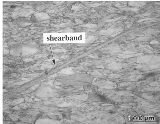
Fig. 8. Adiabatic shearband in a sample strained to  $\gamma = 70\%$  at 296 K initial temperature and 3500/s strain rate.
