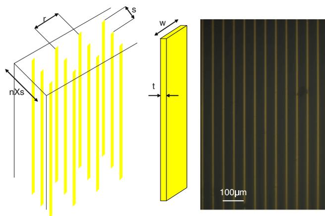
FIG. 2. (Color online) The micron-scale thin strip array. Left: The slab of  $n$  rows of strips spaced  $r$  in-plane and  $s$  through the thickness. Center: A single strip of width  $w$  and thickness  $t$ . Right: Optical micrograph of an array of thin gold strips in PDMS.
