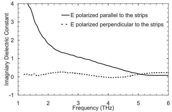
FIG. 7. The extracted imaginary part of the dielectric constant. The real parts are shown in Fig. 5.
